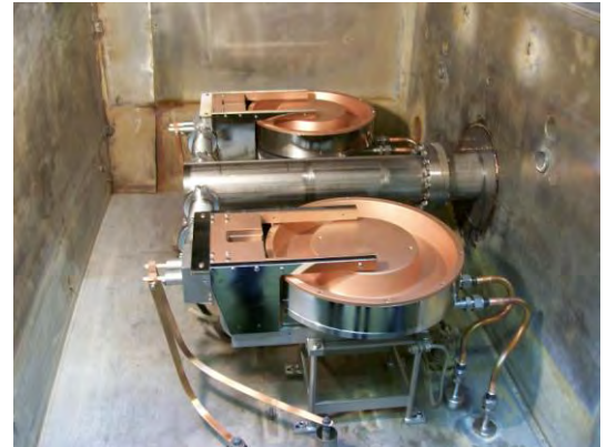
Dual ICR Installation with optional differential pumping
