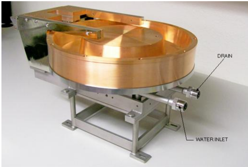
Model ICR water-cooling connections
