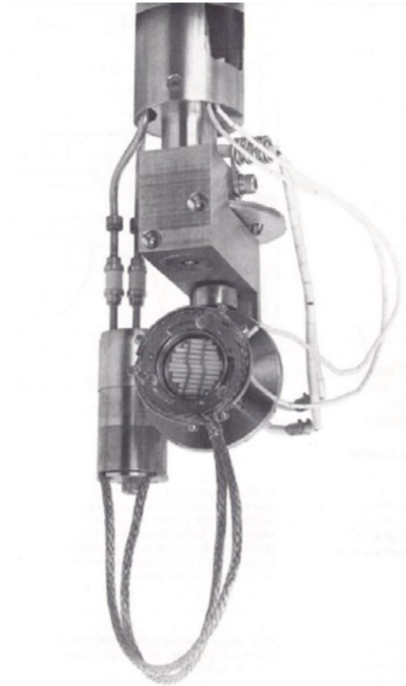
SMR (shown with 1" sample heater, LN 2 cooling, electrical isolation and GB-7 gearbox)
